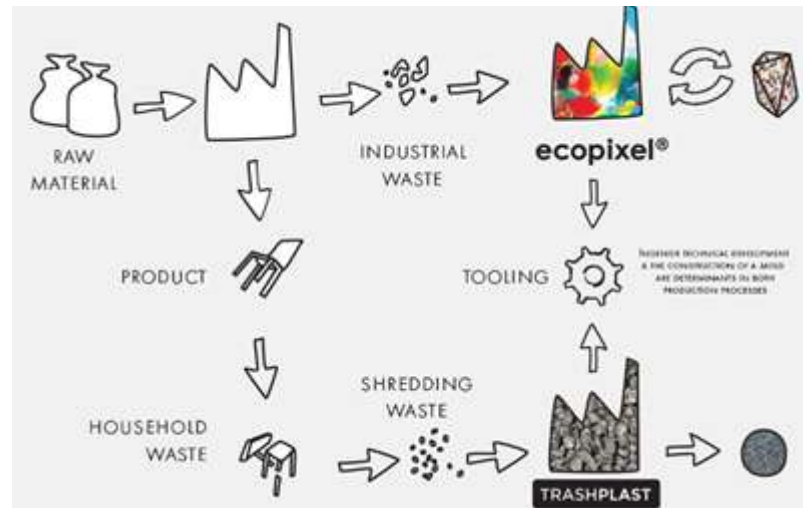
Figure 35. Ecopixel technology. Image source: Ecopixel
